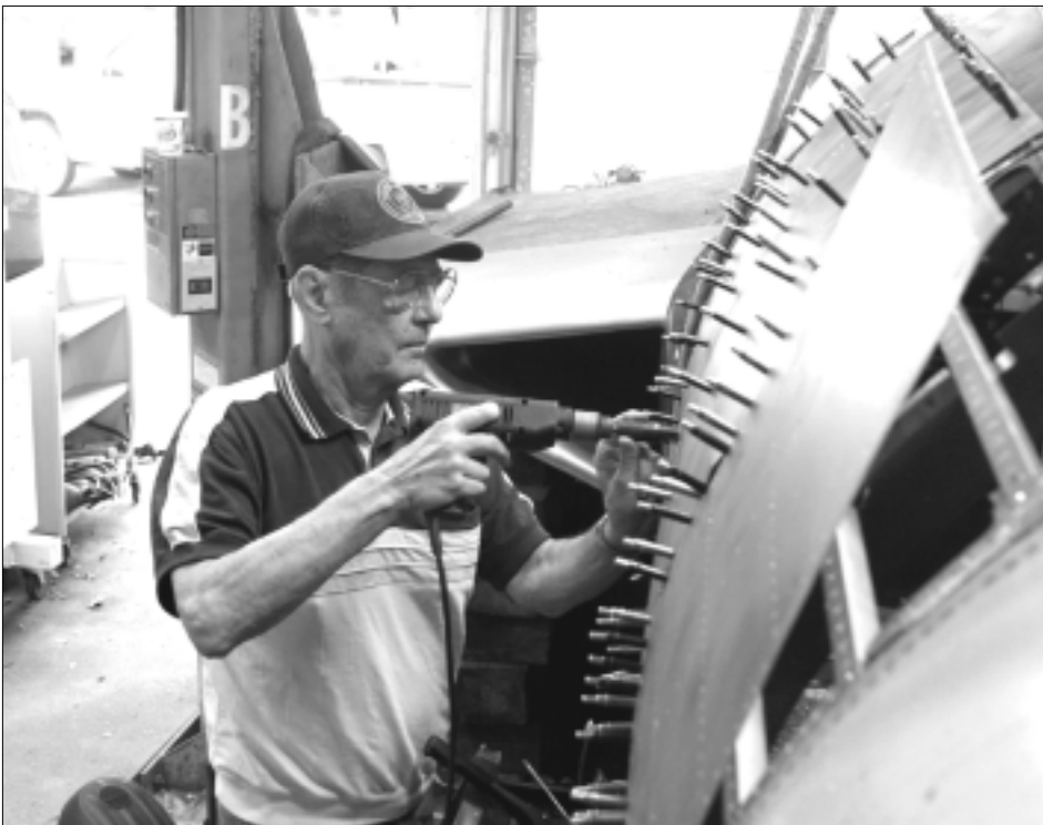
Riveting a new piece of sheet metal on the Panther's fuselage.
